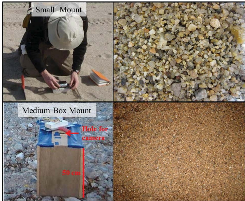
Figure D-1. Left: small and medium grain-size photo mounts used for digital analysis of grain size; Right: photos of bed material taken with those mounts.
