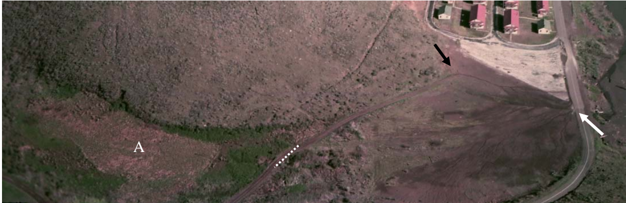
Figure 6. Ca. 1980 oblique airphoto. North and upvalley are to the left. Note the transverse road and headwall crossing (white dotted line), and large rectangular zone (A) in what is now perennial wetland that in the photo appears dry and surrounded by green-vegetated, linear-edged features that may be remnant drainage ditches. Note also that the transverse road ends near the black arrow and the drainage pattern below it suggests that a ditch running along the road conveyed water to this point. The larger drainage network, across the bare area that is now the gravel parking lot, drains to a low point marked by the white arrow, roughly in the same location as the natural drainage seen in Figures 3 and 4.
