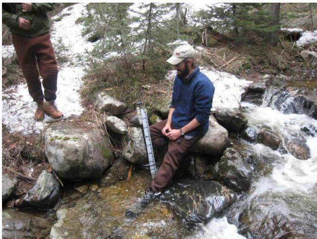
Figure 2. Staff plate mounted to PVC pipe housing pressure transducer, Sawmill Creek reference reach (6/4/09).
