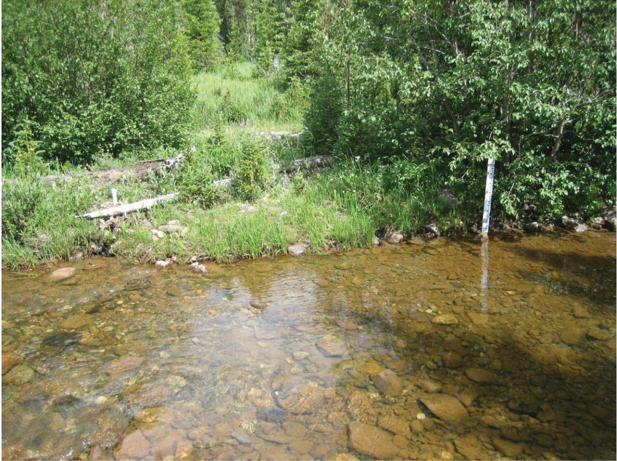
Figure 2: Photo of Shipler Park onsite reference site. Demonstrating groundwater well and staff gage placement for water table monitoring.
