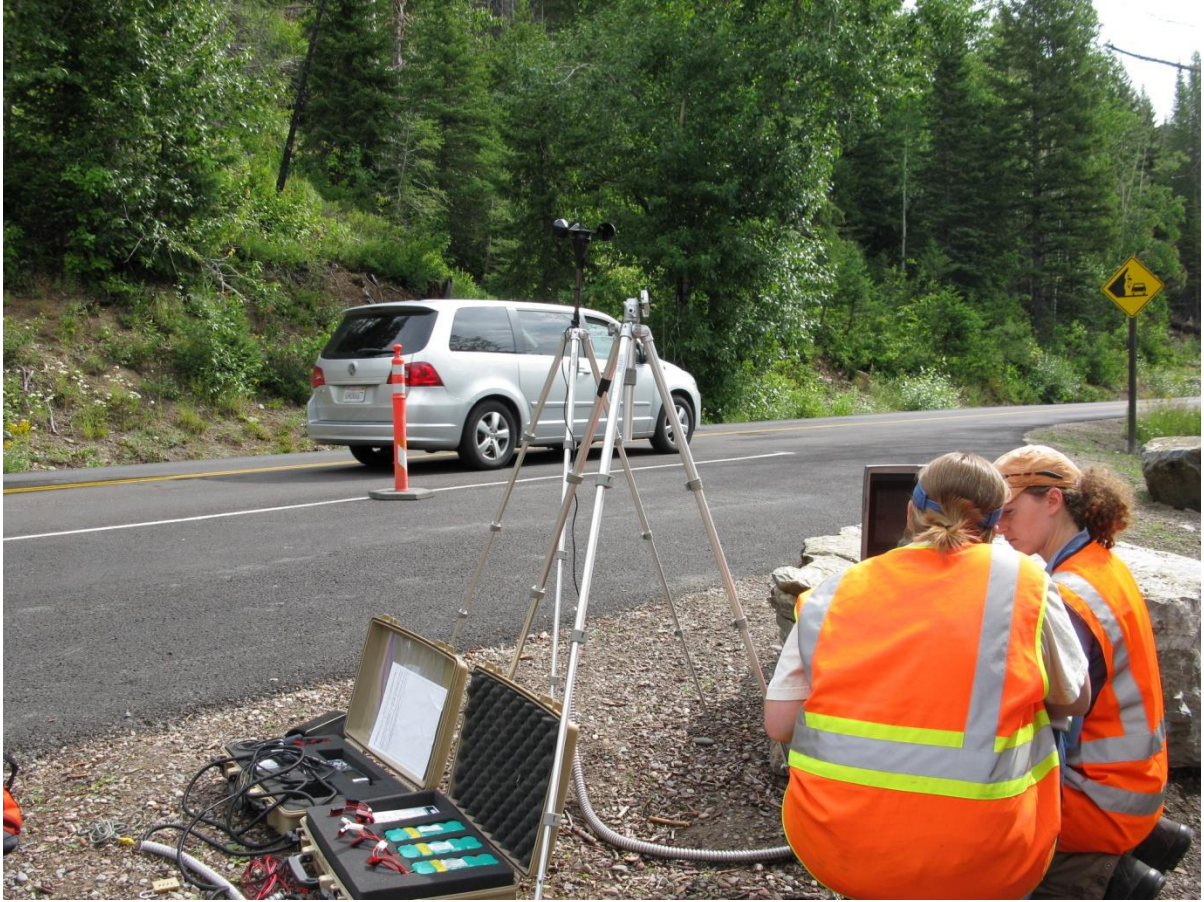
Figure 1. Data collection (sound pressure level measurement and traffic counts) on Going to the Sun Road, Glacier National Park
