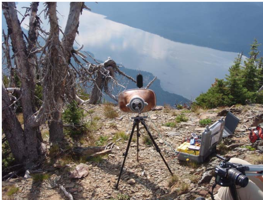
Figure 3. Acoustical monitoring equipment, set up on Mt. Brown, above Lake McDonald (s1)
