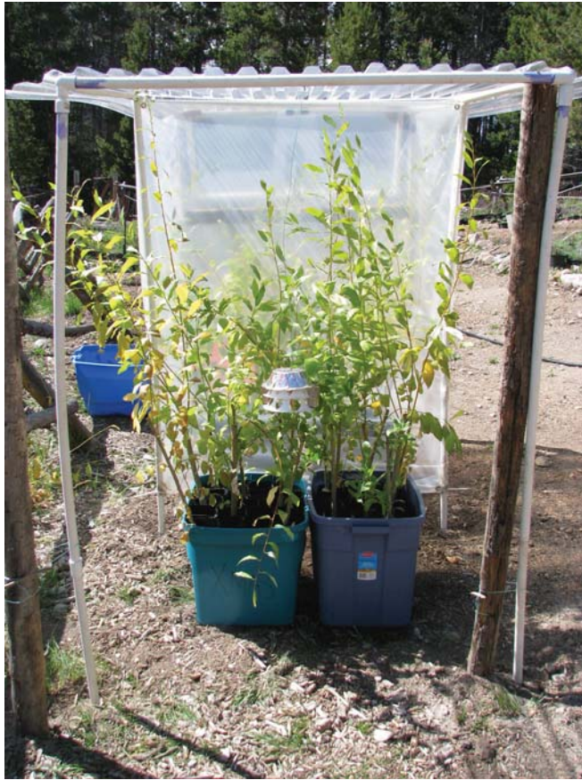
Figure 4.2: One replication of paired experimental treatments: Ambient temperature in front, passive warming shelter in plastic sheeting behind. Hobo (Campbell Scientific) temperature sensor hanging in center.
