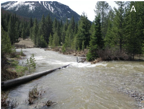
Figure 6. Repeat photographs from Gravel Beach Cross Section on 6/7/10 (A), and 8/29/10 (B) showing formation of a scour hole during high flow due to a log abutting the staff plate. Erosion beneath the gauge reached a maximum of 20 cm on 9/24/10. View is downstream.
