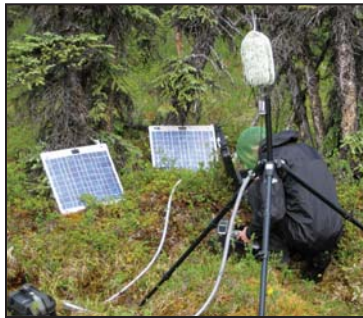
Checking sound equipment set up near the McKinley Bar Trail. Sound clips from continuous recordings will be used in the second phase of the study.
