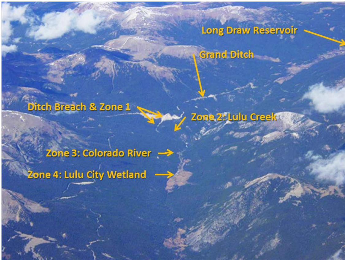
Figure 2. Oblique aerial view looking north up the Colorado River Valley. The Grand Ditch is the tan horizontal line to the middle right of the image and extends to where the Ditch meets Cache la Poudre Pass. The 2003 Ditch breach is located at the arrow that bisects the Ditch, with Zone 1 on the hillslope below. Additional arrows identify Zones 2 (Lulu Creek), 3 (Colorado River), and 4 (Lulu City wetland). Long Draw Reservoir is just off the image at upper right.
