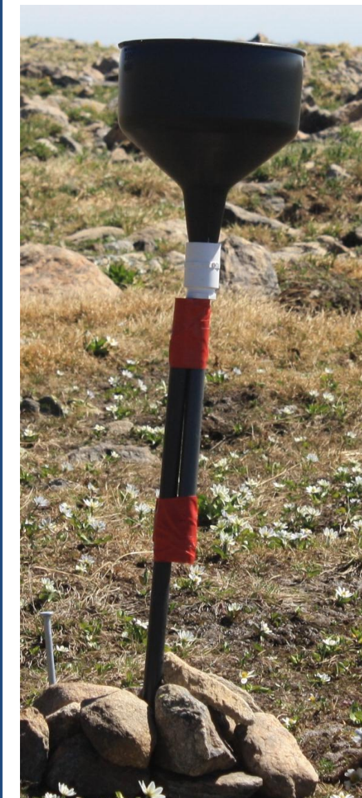
Figure 2. Passive ion-exchange resin column sampler measuring N deposition at Niwot Ridge LTER
