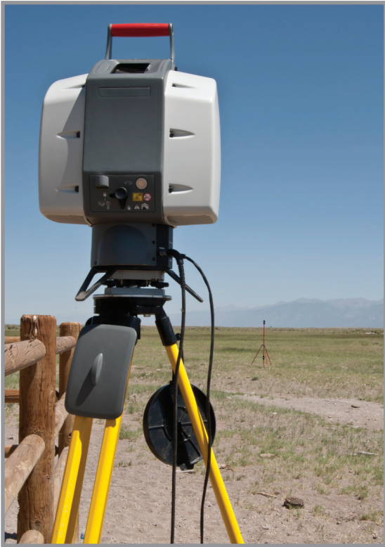
Scanner acquiring HDS target in the background
