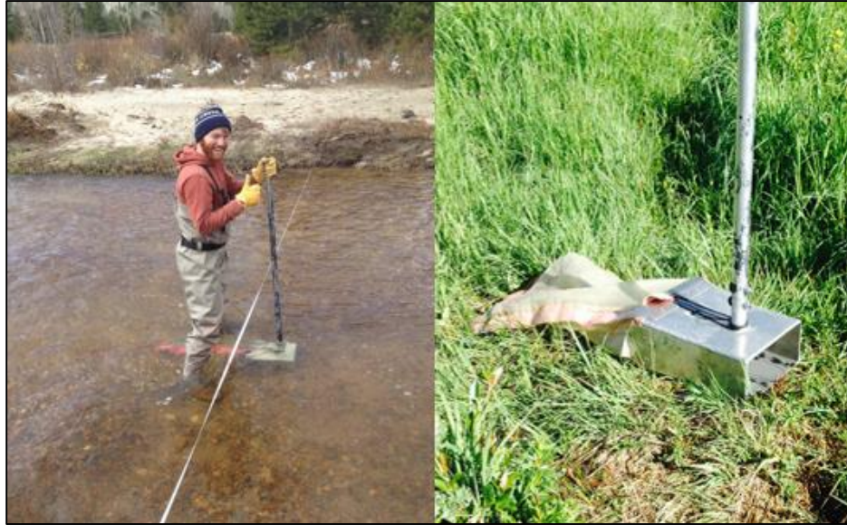
Figure 2.7. Typical bedload sampling procedure with Elwha sampler, shown at FR 1 (left), and close-up of Elwha sampler (right)
