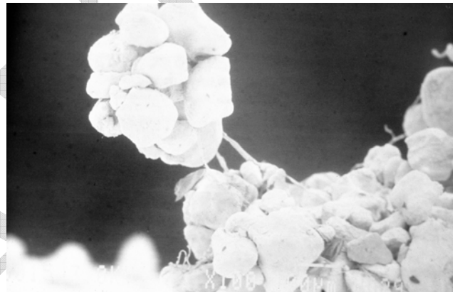
Figure 2. Two photos showing binding of soil particles by cyanobacterial sheaths.
