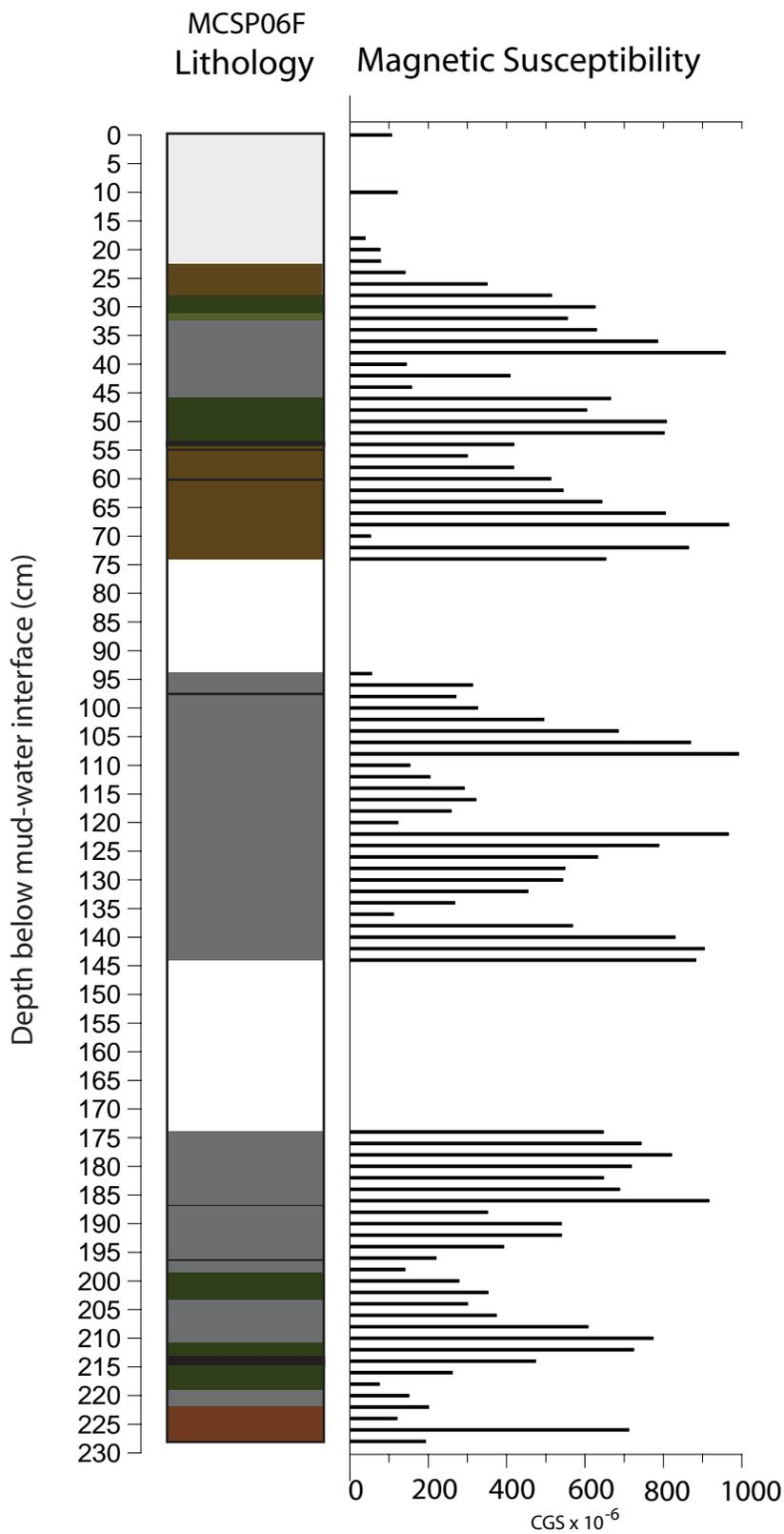
Figure 5. MCSP06F lithology and magnetic susceptibility measurements (see Figure 4 for lithologic descriptions)
