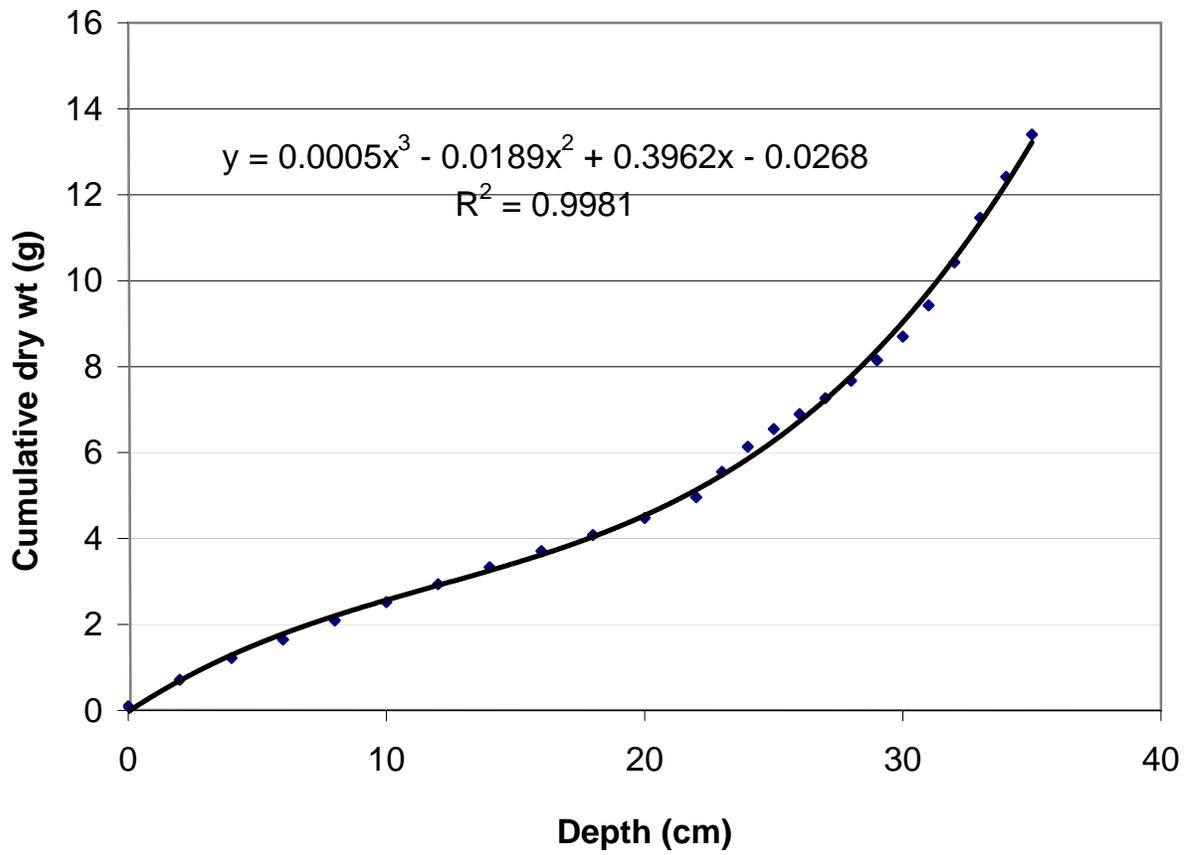
Figure 6. Cumulative dry weight (g) of sediment in core MCSP06D. Note inflection in sediment accumulation rate at 22 cm depth marking the base of the uppermost clay unit.
