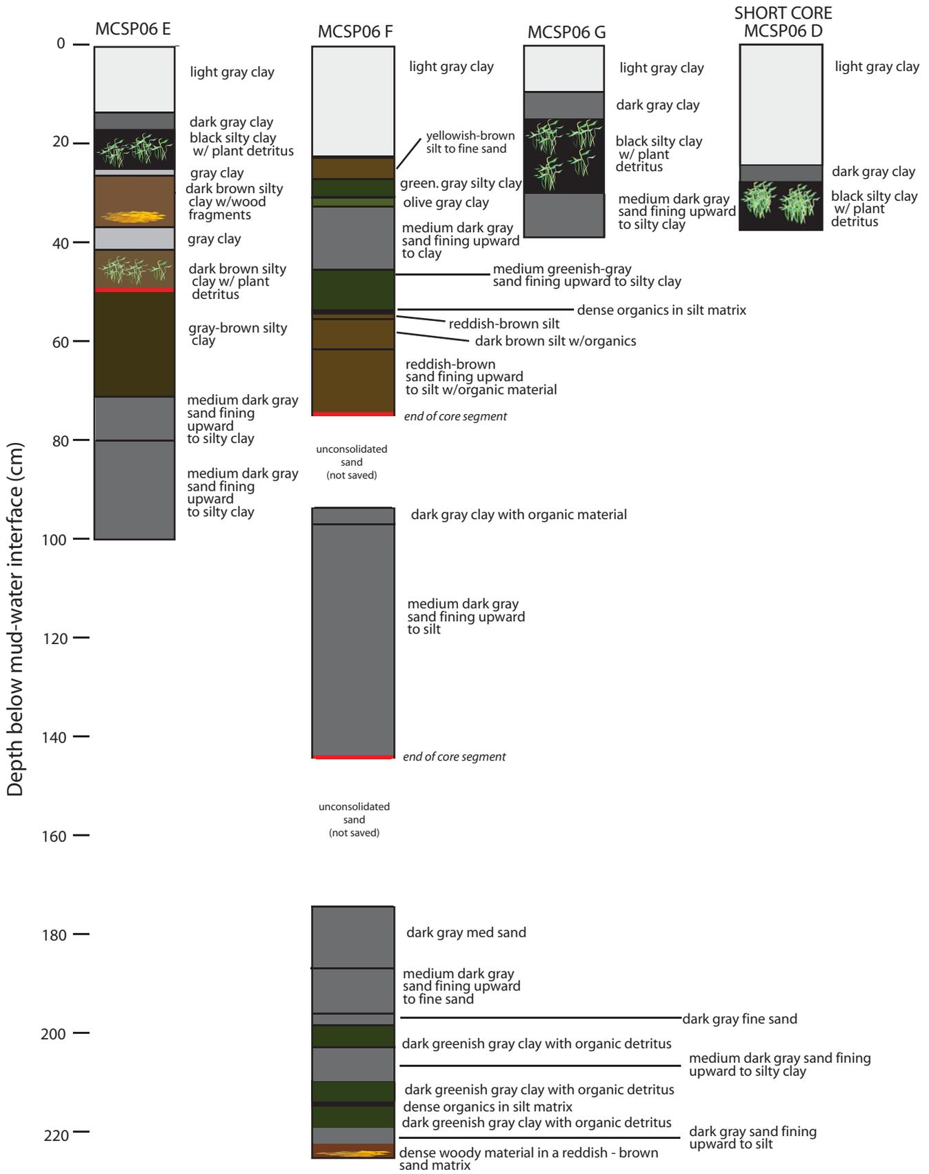
Figure 4. Description of sediment cores from Mammoth Crystal Springs Pond. MCSP06E, MCSP06F, MCSP06G were taken with a Livingstone piston sampler. MCSP06D was taken with a Klein gravity corer. Note that MCSP06F is based on lab descriptions, whereas the other cores were described in the field.
