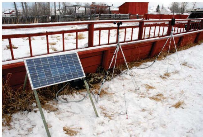
Figure 3: Acoustical monitoring site equipment deployed at GRKO on 17 March 2009.
