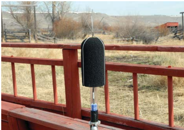
Figure 4: Windscreen (32cm x 10cm) and bird spike enclosing microphone
