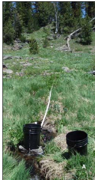
Image 7: RSI setup properly in a small stream, water flowing from right to left.
