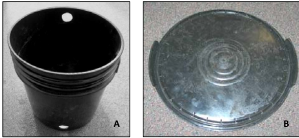
Image 5. A) Bucket with hole drilled into opposite sides. B) Bucket lid with all but two tabs removed; provides easy access into the inner workings.
