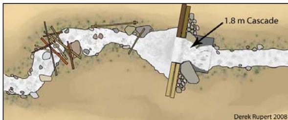
Figure 7: After the barrier and splash pad are completed the water barriers will be removed and the diversion trench will be backfilled. The stream will return to the original channel and flows over the fish barrier.
