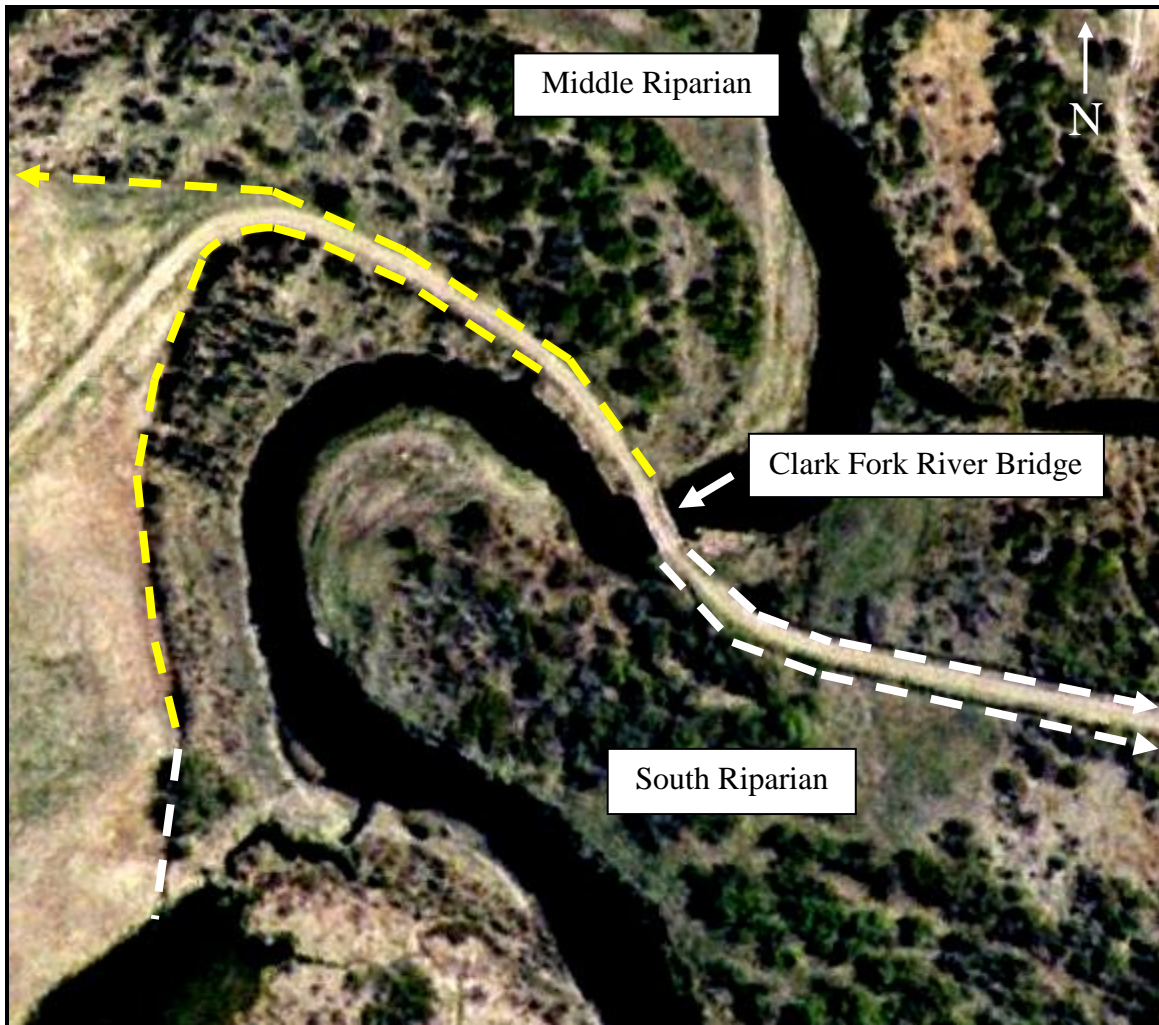
Photo 17. Wood post with woven wire and barbed wire (yellow lines) and jackleg (white lines) fences on the southern boundary of the Middle Riparian area and the north and west boundaries of South Riparian area.
