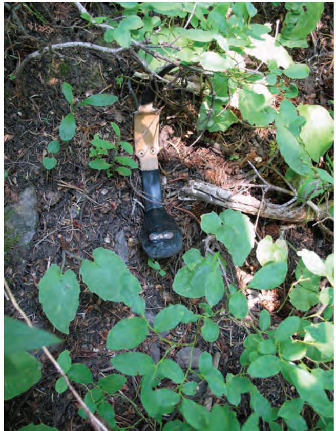
*Left:* Project technician Heather Ristow en route to retrieve a GPS collar in the Absaroka Mountain Range, Montana, 2006. *Right:* A GPS collar as found after its release mechanism fired and the collar dropped.
