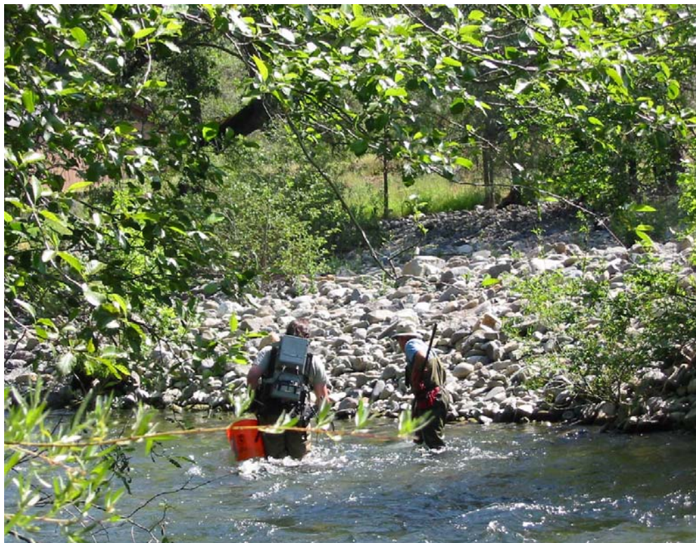
Fig. 9. Collecting fish from Clear Creek using a backpack shocker.
