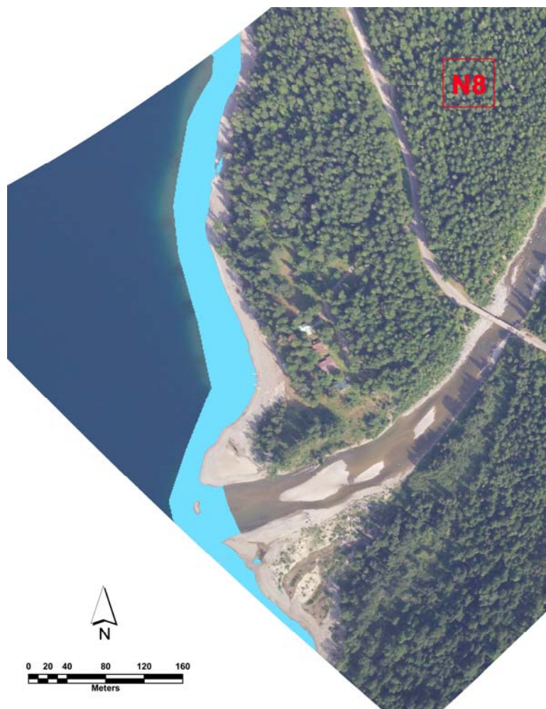
Figure 5. Classified image of Section N8, North Lake McDonald. The shoreline has been analyzed for algal spectral signature. Light blue = no-low algal reflectance, orange = diatom reflectance, red = green algal reflectance.
