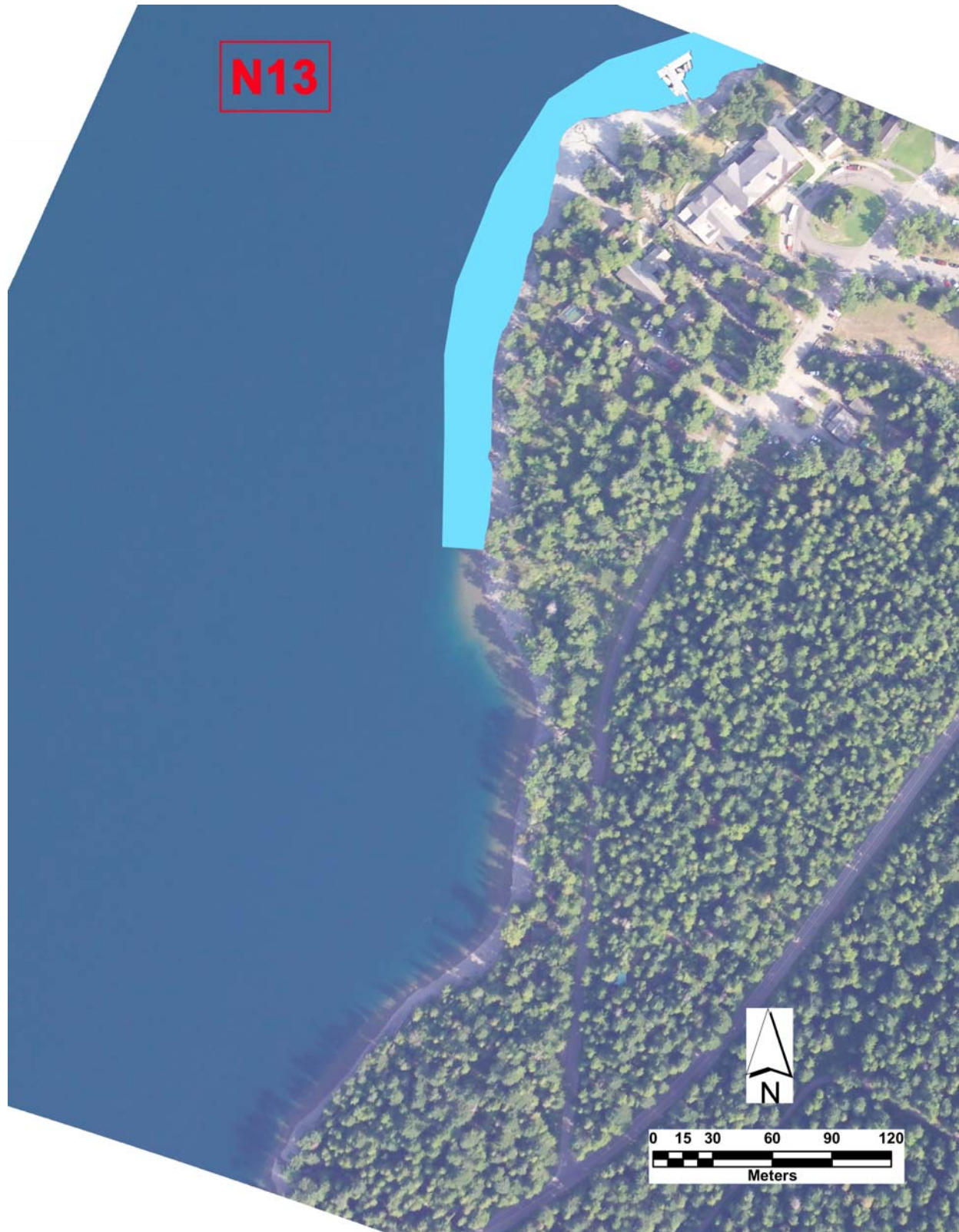
Figure 10. Classified image of Section N13, North Lake McDonald. The shoreline has been analyzed for algal spectral signature. Light blue = no-low algal reflectance, yellow = diatom reflectance, red = green algal reflectance.
