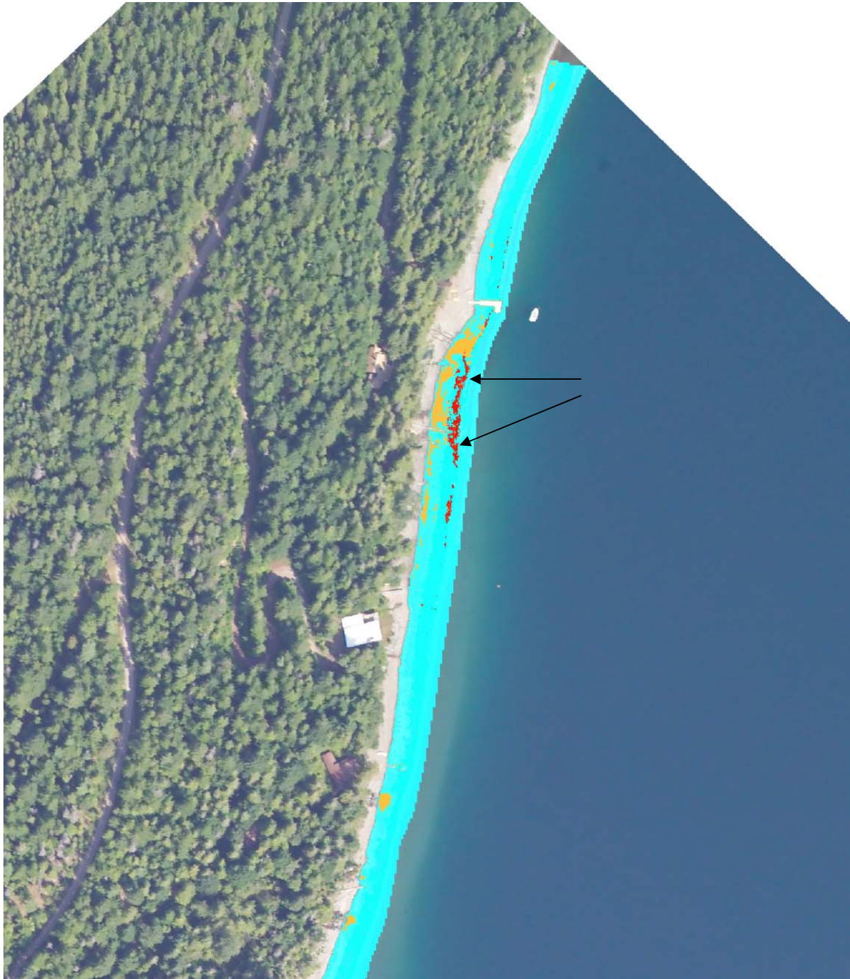
Figure 12. Classified image of northern end of Section S3, South Lake McDonald. The shoreline has been analyzed for algal spectral signature. Light blue = no-low algal reflectance, yellow = diatom reflectance, red = green algal reflectance. See also Appendix A, Figure A3. Arrows indicate sites of increased algal biomass.
