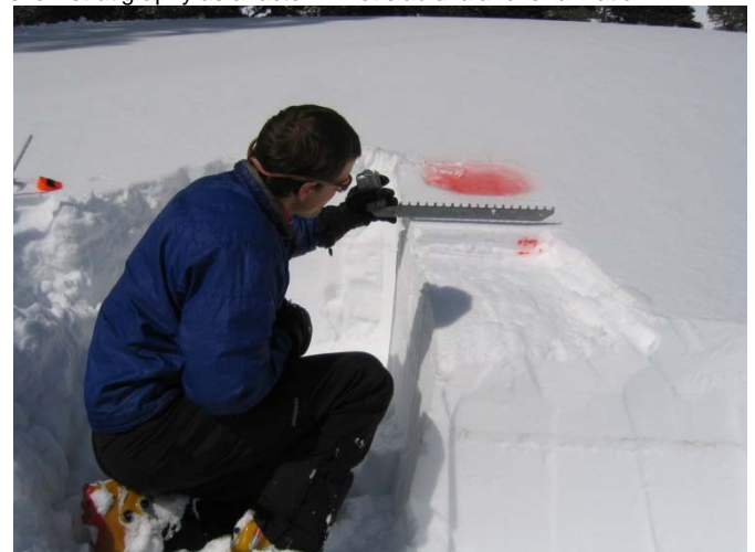
Figure 3: Researcher investigating water flow through the snowpack by using red dye tracer. Photo: Karl Birkeland
