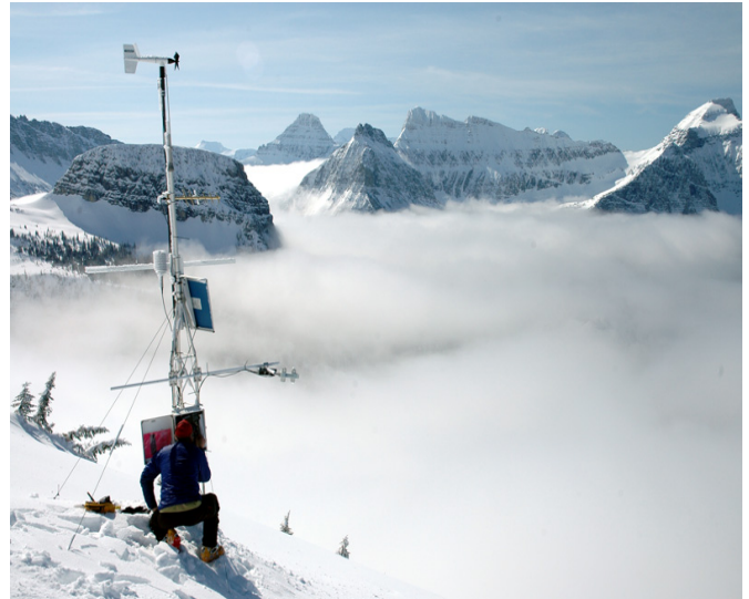
Figure 4: Researcher monitoring meteorological measurements at the Garden Wall Weather Station. The GTSR is located ~2000 vertical feet below and in the clouds in this photo.
