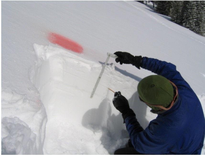
Figure 15: After applying dye, I marked the slope parallel cuts that are conducted 10 minutes after dye application. Photo by Karl Birkeland.
