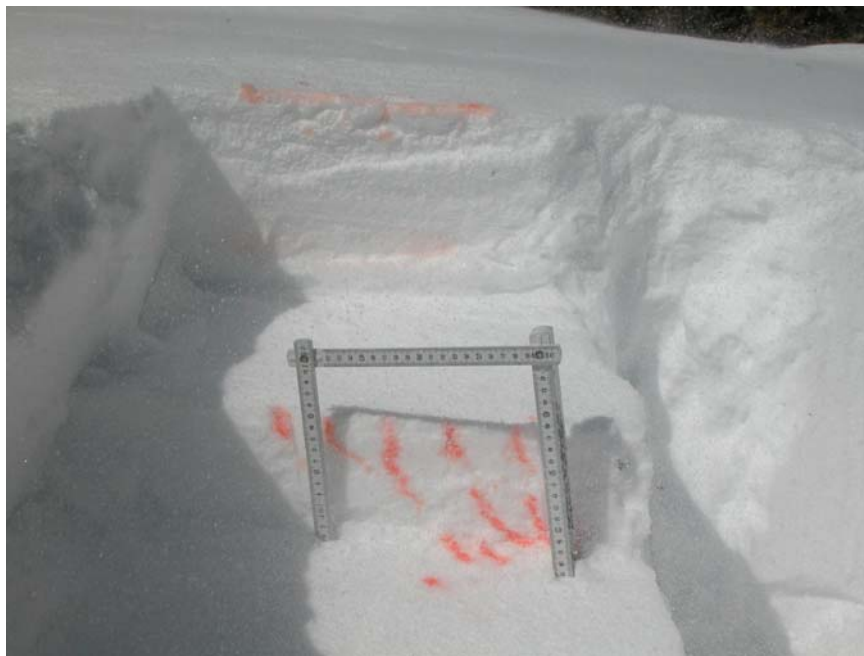
Figure 44: Flow fingers ~30 cm from the snow surface after the top 30 cm was removed to determine the existence of preferential flow. Flow fingers almost always formed when water was added to a dry snowpack except for already wetted snow where preferential flow had previously been established.
