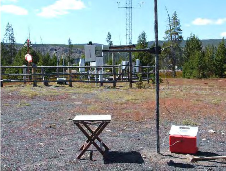
Figure 2. Standard reflectance panel and Exotech 4-band radiometer measuring incoming irradiance from the sun setup in the Upper Geyser basin area during one of the daytime flights in Yellowstone Park.
