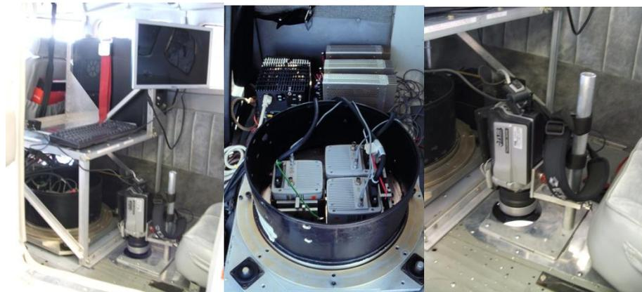
Figure 1 Details of the USU airborne multispectral remote sensing system and FLIR SC640 thermal IR camera installed in the Cessna TP206 remote sensing aircraft.
