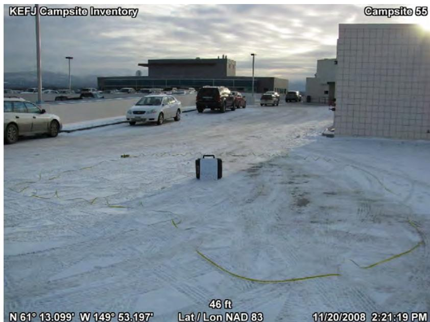
Figure 7 – How an image taken after a Photo\_Pt can be combined in GPS-Photo Link to incorporate the position and field comment. A shapefile is also generated that contains the additional attribute information.
