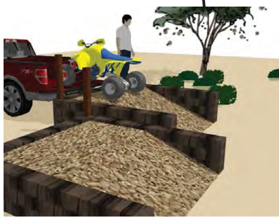
OHV Loading Ramp. Two levels for different height truck beds.
