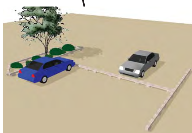
Parking bordered by some type of environmentally friendly material. Individual stalls not marked.
