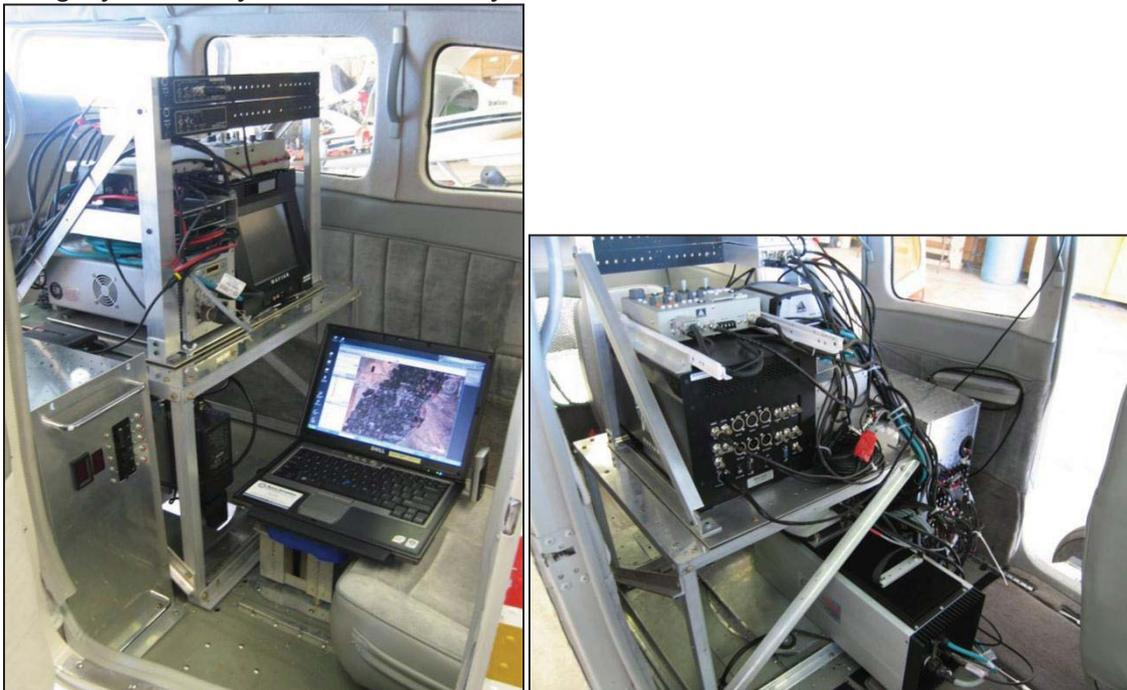
**Figure 2.** The LASSI instrument installed in the USU Cessna TP206 remote sensing aircraft.
