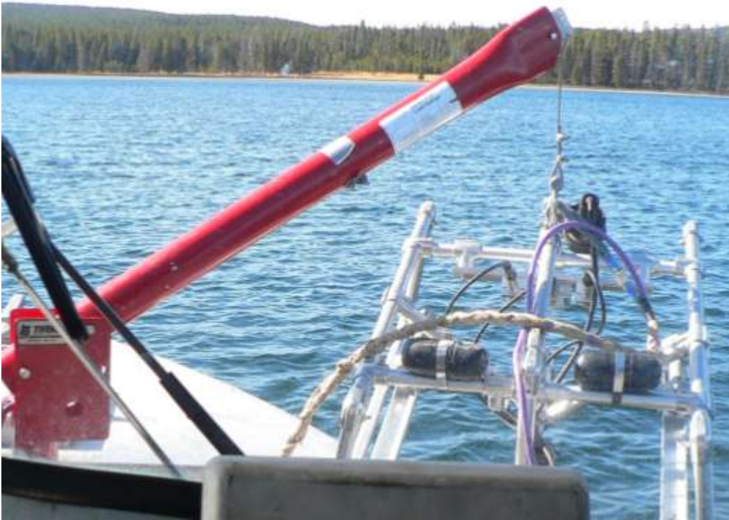
Figure A-3. Deck-mounted winch used to raise and lower the camera/tow sled configuration.
