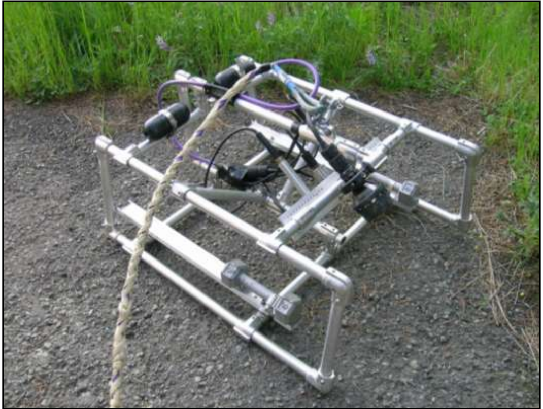
Figure A-1. Towed vehicle with underwater video camera, underwater light, and two laser lights.
