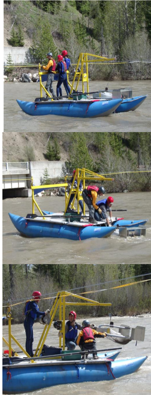
Figure 1. Sampling bed load transport rates on Pacific Creek: (A) moving the boat across the cable using the roller-towers; (B) deploying the sampler; and (C) retrieving the sampler from the bed with a partially filled bag of sediment.
