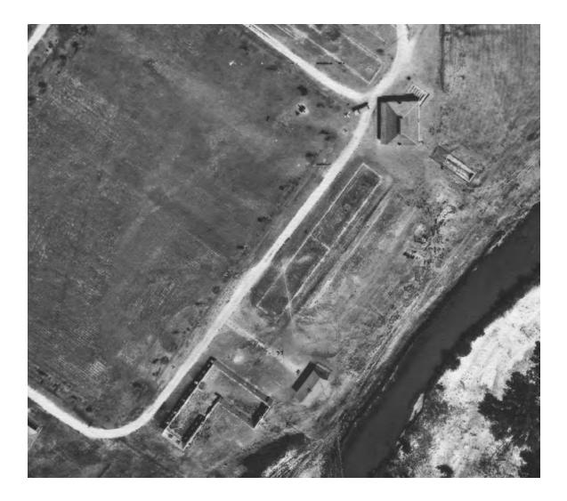
Figure 4: 1996 color infrared aerial photograph of Fort Laramie Parade Ground, showing location and general condition of the 1866 Infantry Barracks. Note erosional area on the southwest corner of the barracks complex, compared with the 1973 black and white aerial photograph. (Courtesy Fort Laramie National Historic Site).
