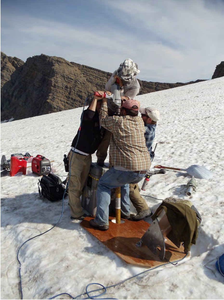
GLAC-38, core 2, showing the difficulty of putting enough pressure on the drill.
