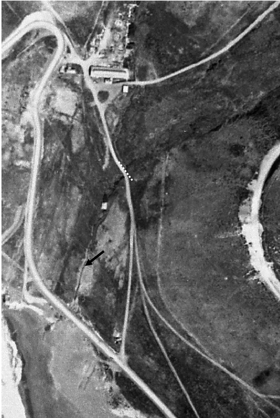
Figure 2. 1940 air photo (north is up). White dotted line indicates the location of the headwall, black arrow indicates a drainage ditch. Note the small building between the arrow and headwall that is visible in figures 3 and 4.
